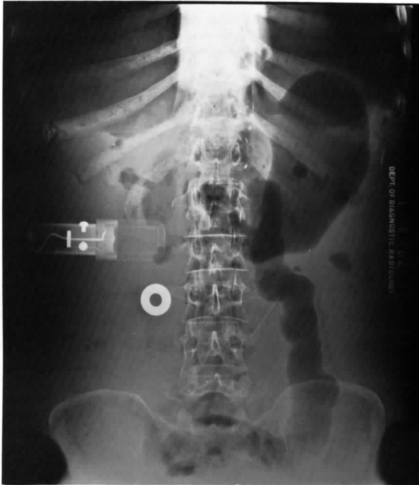
Figure 11.3. Product comparison phantom film. Each image should contain a washer to mark the spot for density matching, lead letter identification information that is not related to the product name, and an ionization chamber for monitoring the phantom entrance exposures. All edge markings are then trimmed from the film so that neither the film nor the screen can be identified by the viewer.
